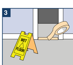
3 Tape off doorways and edges. Place wet floor signs at all entranceways. 10 - 15 Minutes
